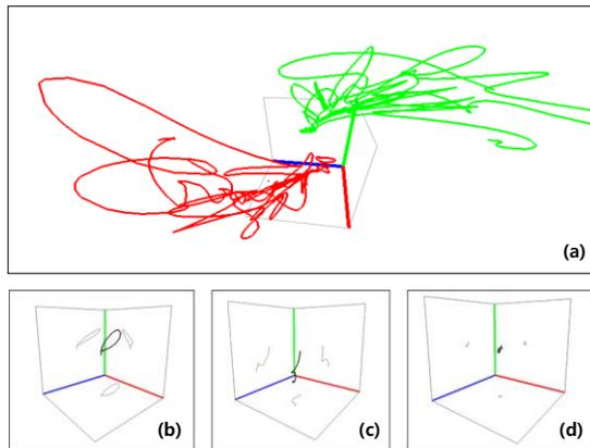
**Figure 3. (a) Traces of the pen with different directions. Different pen-spinning gestures were sensed using a three-axis magnetometer: (b) Charge, (c) Twisted Sonic, (d) Zigzag.**
