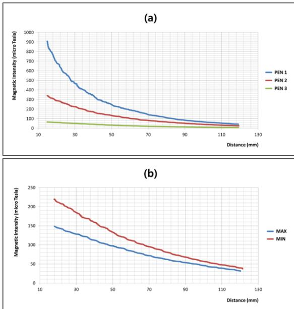
**Figure 4. (a) Graph of magnetic intensities according to the distance for different pens. (b) Graph for two different pressures applied to the pen.**
