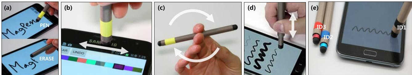
**Figure 1:** Five magnetically driven input techniques for pen interaction: a) detecting pen orientation, b) making a dragging motion along the device frame, c) determining pen-spinning gestures, d) estimating the pressure applied to the pen, and e) identifying
