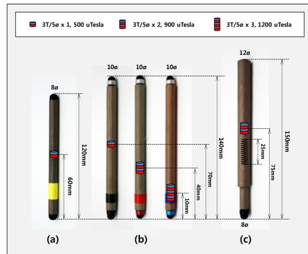
**Figure 2. Three types of *MagPen* prototypes: (a) a simple pen, (b) three identifiable pens, and (c) a pressure-sensitive pen**
