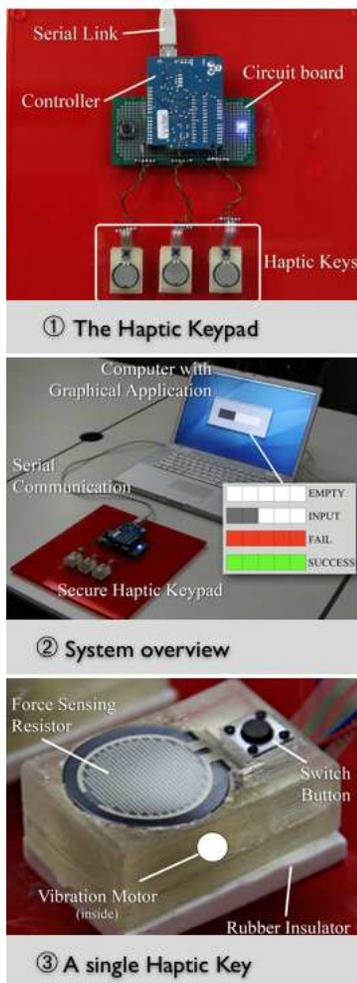
**Figure 1.** The *Haptic Keypad* system, an overview of how it is interfaced to a computer and a close-up of a key.
