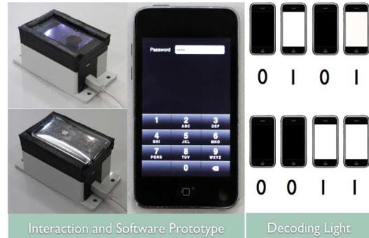
**Figure 2** LuxPass receiver unit prototypes (left) and software GUI. Simplified example of light encoding (right).
