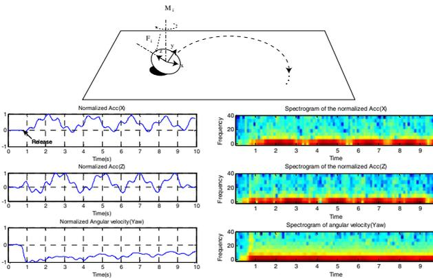
**Fig. 3.** Example of erratic motion triggered by initial force ( $F_i$ ) and moment ( $M_i$ ) provided by the user. Resultant motion signal in the time domain and the corresponding spectrogram shows that two or more frequency components dominate.
